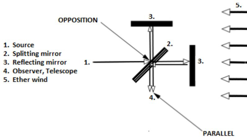
**Figure 3.20** MMX with an Ether Wind
