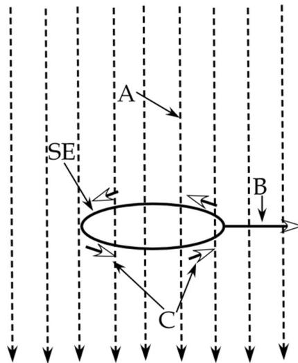
**Figure 3.33** Sagnac Interferometer
