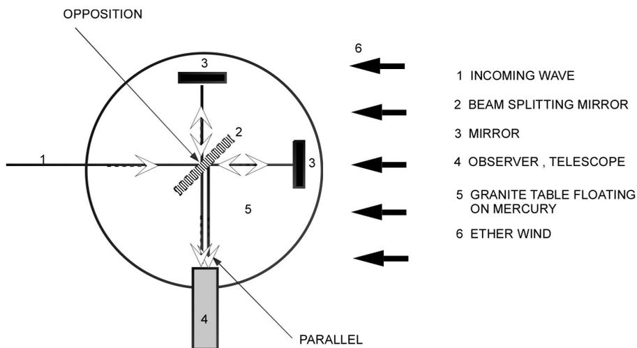
Figure 3.17 MMX with an Ether Wind [Fair Use]
