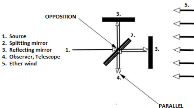
**Figure 3.18** MMX with an Ether Wind
