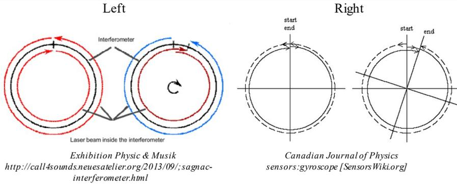
**Figure 3.32** Fiber Optic Sagnac Interferometer [Fair Use]
